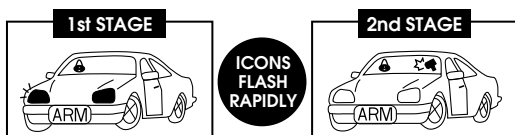
FIG-5: Pager LCD Icon Change Upon Shock Detection
